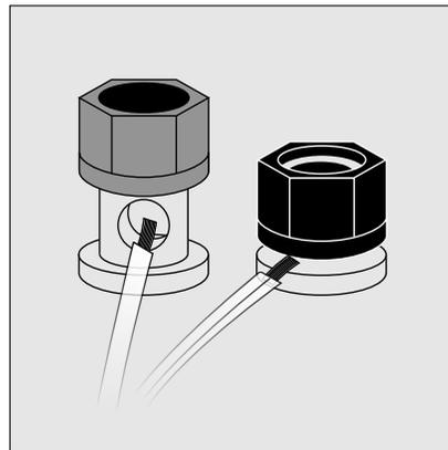
Using the gold-plated binding posts: you can easily connect banana-plugs, spade-plugs and bare wire. Insert the wire into the hole tighten securely (do not let bare wire hang out side of hole).
