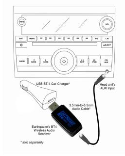
Designed with convenience in mind, the BT4 features fast and easy device pairing method and over 10 meters of open space wireless range. It can remember up to 7 paired devices and will also auto reconnect to the last paired device if it is within range. Full audio frequency bandwidth 10Hz to 20kHz.
